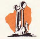
Hot drop forging produces strength and durability not achieved by any ather method. This is the first step in the fabrication of all WISS products—and a basic reason far their long life and satisfactory performance.
